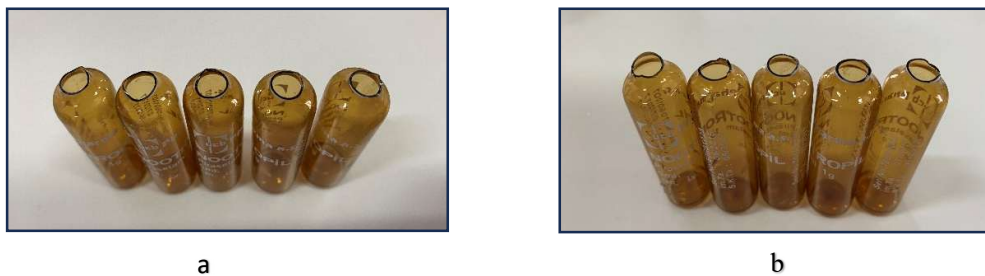
Fig. 2. Broken states of the ampoules, a; without using apparatus, b; using the apparatus
